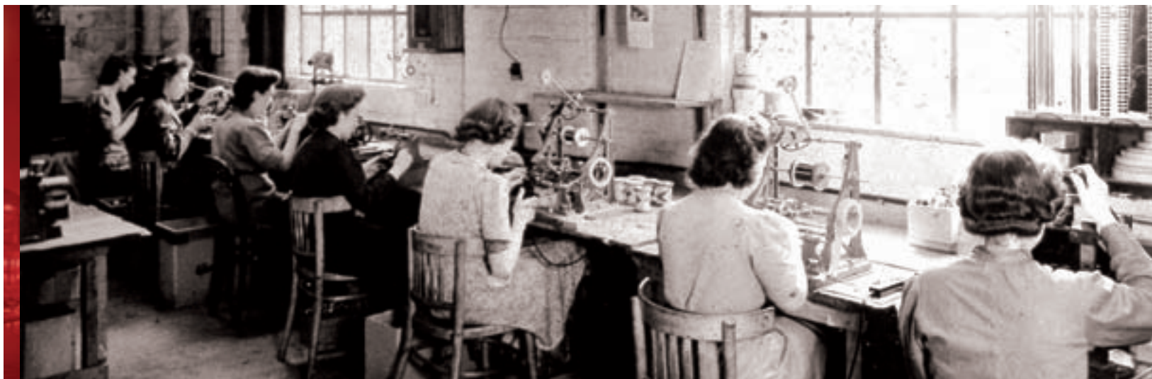
Winding coils for Marconi transformers kept the 20 staff busy throughout the war.
